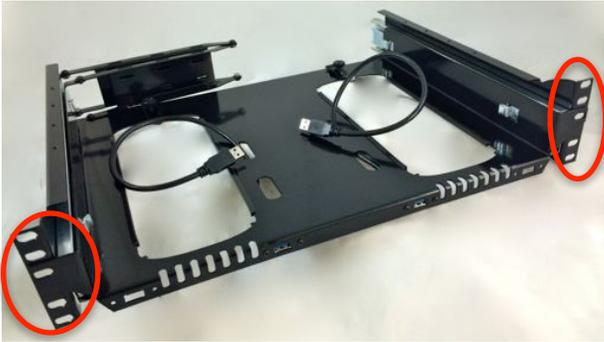
Mount the empty MPR-2X into a 19" rack enclosure with the provided 10-32 rack screws. The MPR-2X will be 4U spaces tall when the Mac Pro is installed so be sure to mount the unit so that it is at the bottom of the available 4U space. Do not use the mounting hole in the middle, reserve that one for the thumb screw. The thumb screw will secure the sliding feature so that the unit stays locked in the rack.
