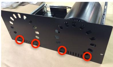
The optional MPR-BP can be added to provide a finished look as well as control airflow. Mount the plate to the USB cable mounting holes with the included 6-32 self threading screws. If you ordered your unit with the optional USB cables, use the mounting screws for the cables to attach the plate. On the side of the plate you will see holes that allow the thumb screws to be used for quick access to the sliding feature of the rack.
